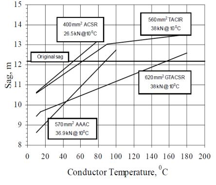
**Next step:** conductors with "knee point" to reduce the increase of sag with temperature Temperatures up to 250° C
