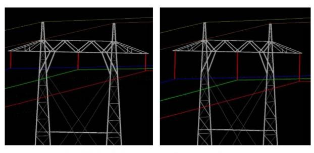
Figure 7. Left: The line before uprating. Right: First proposal for uprated line.
