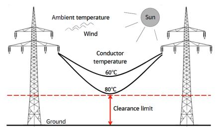
Figure 1: Clearance depending on ambient conditions and current
